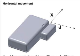
X = +/-5 mm, switching distance 20 mm < d < 30 mm X = 30 +/-5 mm, switching distance 7.5 mm < d < 15 mm
