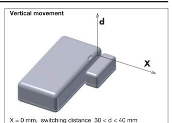
X = 10 mm, switching distance 25 < d < 35 mm X = 20 mm, switching distance 15 < d < 25 mm
