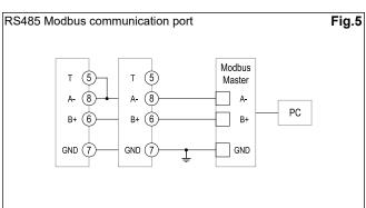
Additional instruments with RS485 are connected in parallel. The serial output must only be terminated on the last network device connecting terminals A- and T. For connections longer than 1000 m use a signal repeater. Maximum 247 transceivers on the same bus.
