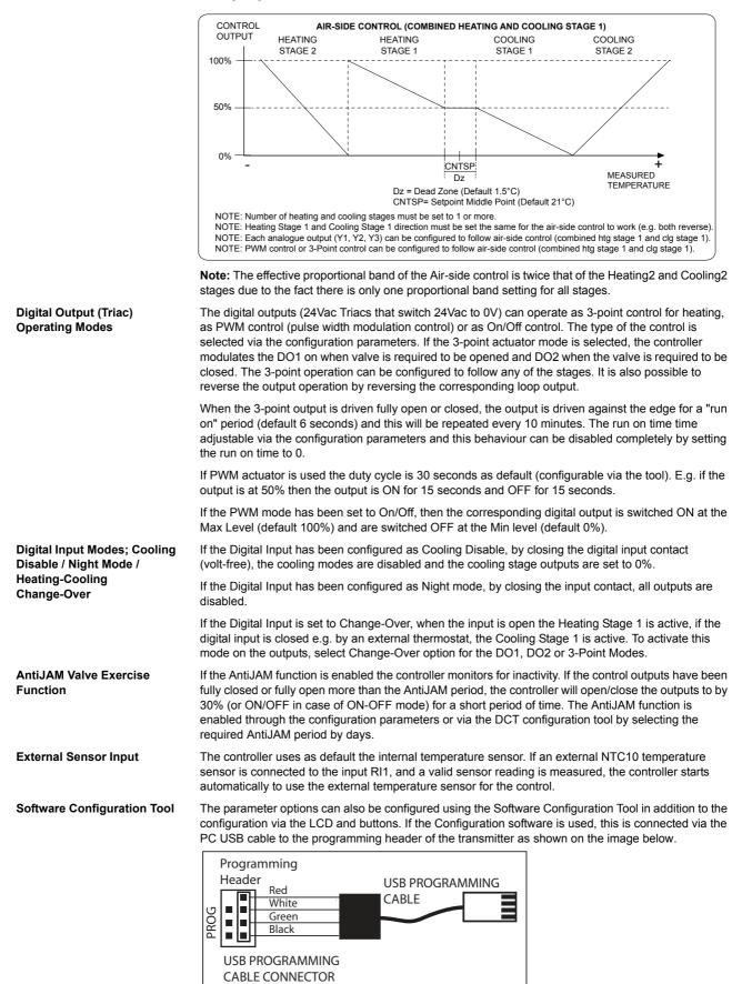
The correct process for connecting the controller via the USB is as follows:-
