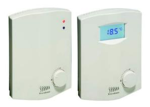
models, the display shows the heating and cooling modes, the current active actuator position, and the current temperature reading. When the setpoint is adjusted, the backlight is switched temporarily on and the current setpoint is displayed. The controllers have built-in Modbus RS-485 communication for connection to BMS systems.
