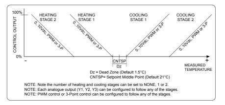
Between heating and cooling stage 1 is a control deadband. This prevent rapid switching between heating and cooling. The deadband is adjustable in the configuration parameters.
