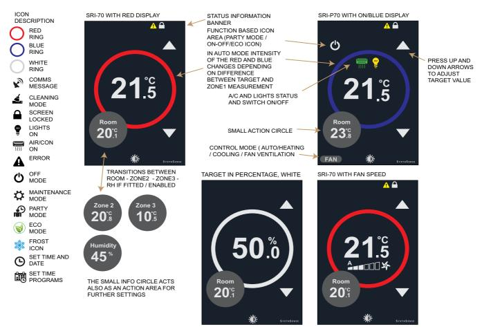
The SRI-70 room interface home screen has four touch sensitive areas that allow the system settings to be altered. All parameter values are available as Modbus/BACnet network variables. Fan speed and setpoint are available as 0-10Vdc outputs with SRI-71.
