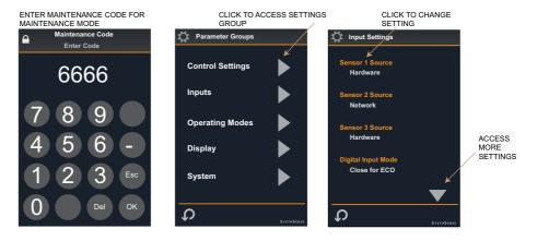
The SRI user interfaces are configured to operate in different modes via the configuration parameters accessible through the maintenance mode.
