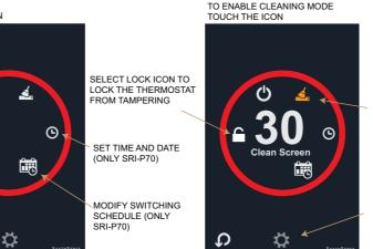
SELECT CLEANING ICON TO ENABLE CLEANING MODE. THE DISPLAY WILL COUNT DOWN FROM 30 SECONDS DURING WHICH ALL BUTTONS ARE DISABLED ALLOWING SCREEN CLEANING.
