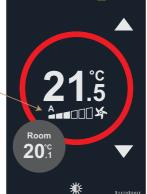
'A' IS DISPLAYED WHEN UNDER AUTO-MATIC CONTROL (NETWORK), IF FAN MANUAL MODE PARAMETER HAS AUTO OPTION SELECTED.
