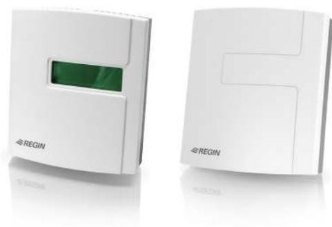
A range of room transmitters for measuring carbon dioxide concentration in indoor environments. The transmitter has a built-in CO<sub>2</sub> sensor with output signal 0...10 V, a PT1000 sensor with separate terminals, as well as an output signal for relative humidity.
