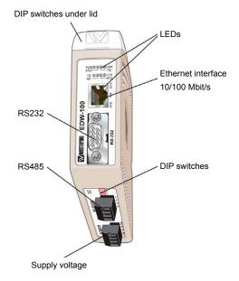
ConverterTCP can be installed on a DIN rail and features two communication ports; one RS485 port and a TCP/IP port.
